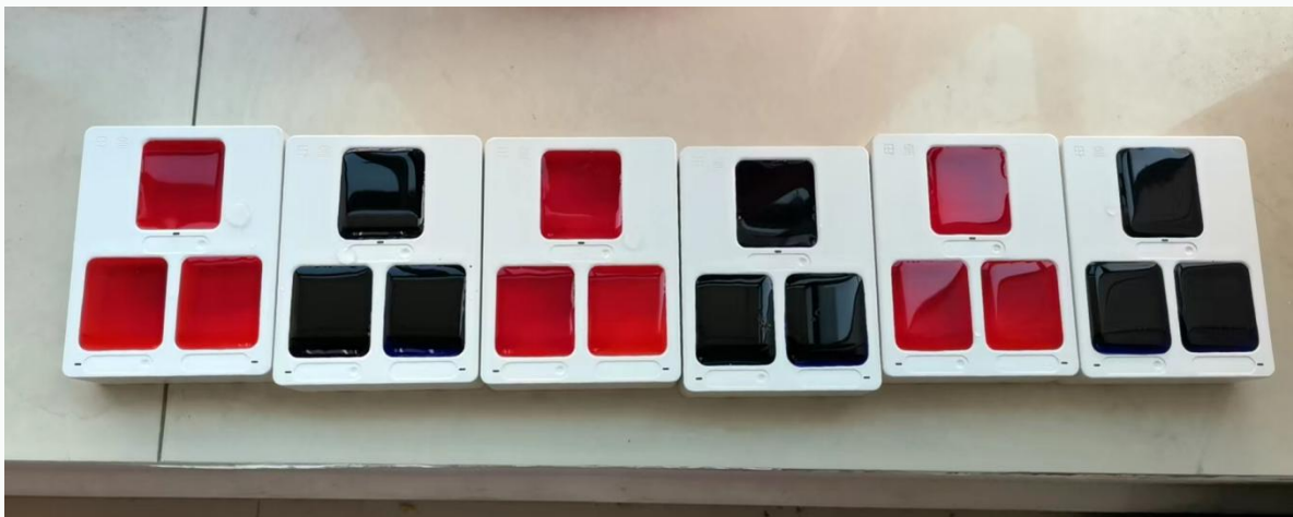
Seepage test (渗水测试)
